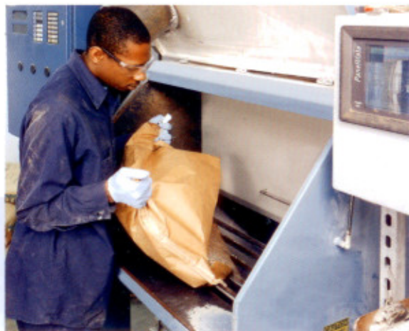
A negative-pressure feed hopper is used for the manual addition of small quantities of ingredients to the mixer.
