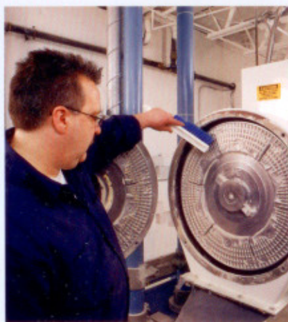
The interior of the attrition mill is easily accessible for cleaning and maintenance.
