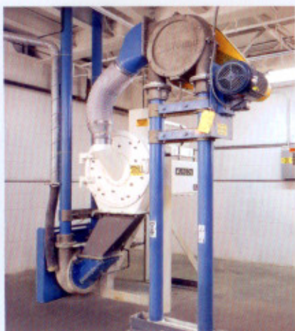
Fine powders are processed in the attrition mill and pneumatically conveyed to the packaging area.
